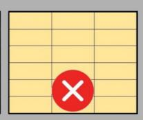
SPC tiles should be installed with staggered joints as shown in the two examples above
